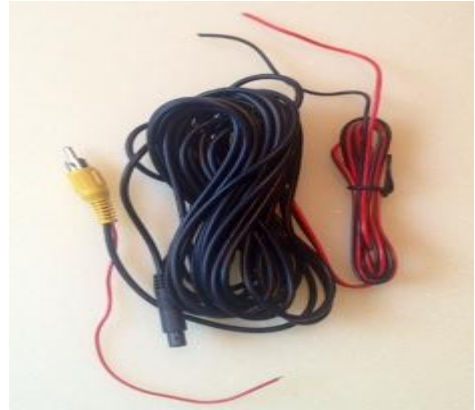
Video line, power feed for camera and back power feed to DVR screen for reversing camera.
