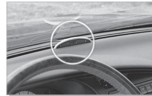
2 side, 4-colour digital LED indicator with built-in buzzer
