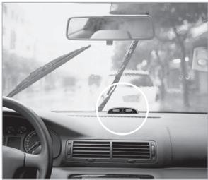
2-color digital LED display with built-in buzzer
