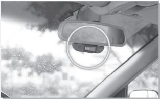
3-colour LED indicator with built-in buzzer
